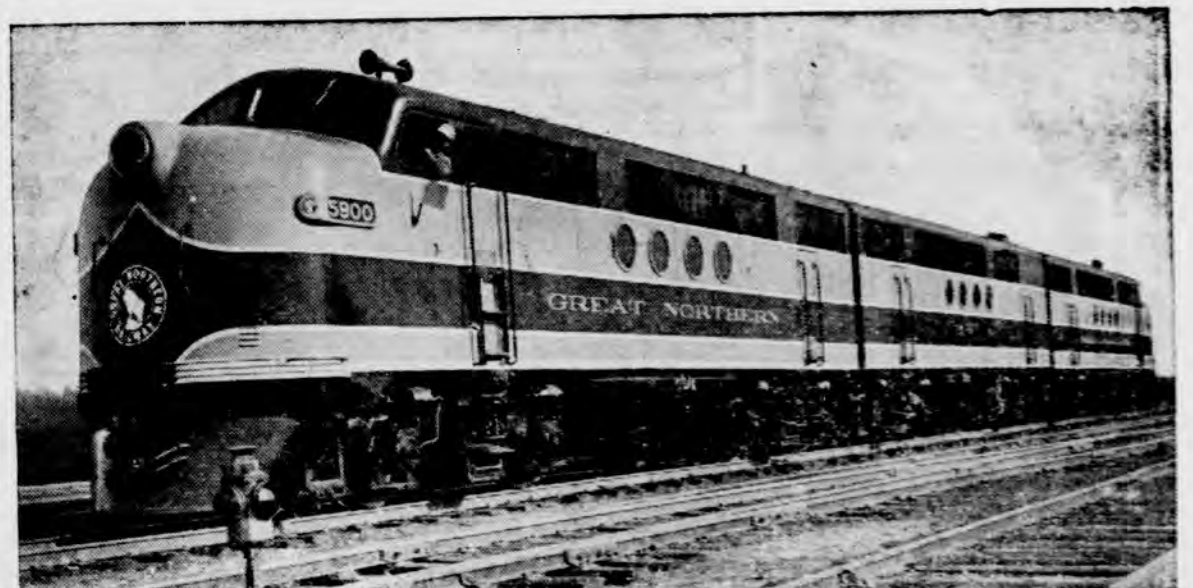
Expediting heavy freight and passenger trains across the Rocky Mountains is the job of this new three-unit Diesel-electric engine. Its 4,050 horsepower is assurance against "bottlenecks" in the Rockies.
