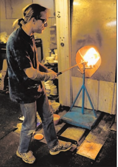
Richard Lowrie feeds a glasswork in progress through the “glory hole” of his propane-fed furnace. Heating the piece periodically in this 2,300-degree furnace helps to keep the glass pliable.
