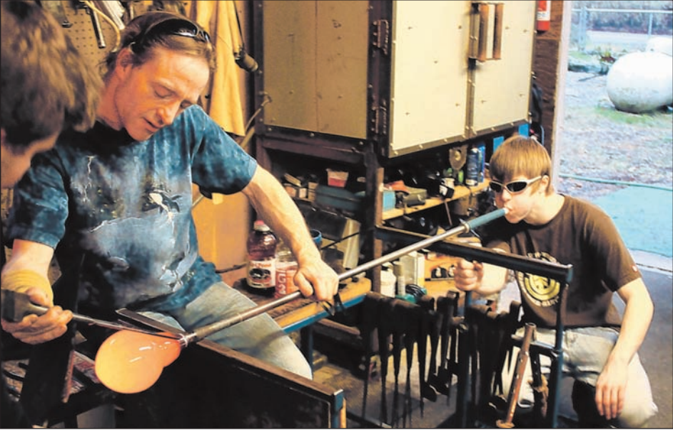
Glassmaker Richard Lowrie begins to shape a piece using a jack tool, while his son, Levi, 19, blows on the opposite end of the blow pipe, which holds the molten glass. The air pressure gently expands the glass. “A lot of the tools, like the jack, have been in use for 2,000 years,” says Lowrie.
